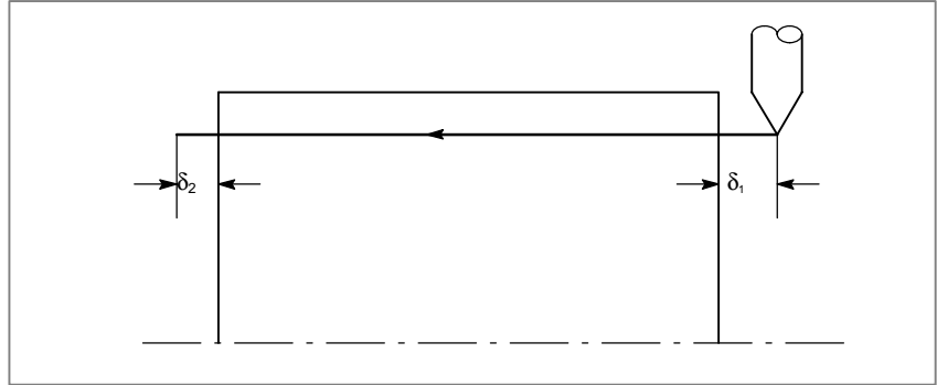
Fig. D.1 (a) Incorrect thread position
